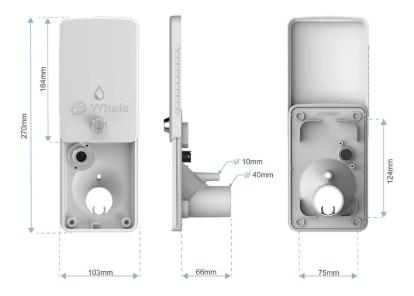
Unique 2 in 1 design includes a 12V pump power supply and Motorhome fill all in one socket. The secure hose clip keeps the pump in place during filling. The Motorhome Filler + 12v Power Socket incorporates a lock to protect your water supply and a vent pipe ensuring the tank is vented at all times, preventing airlocks. This socket is suitable for use with any standard hose and is to be used with cold freshwater only.
